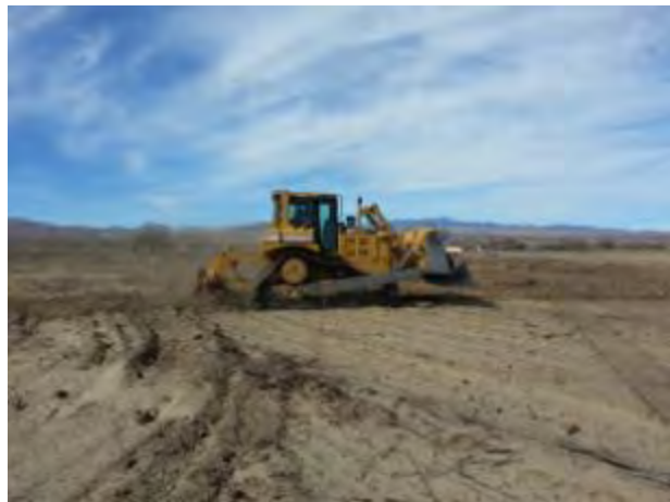
Bulldozer pulling the root plow through the soil, February 2016
