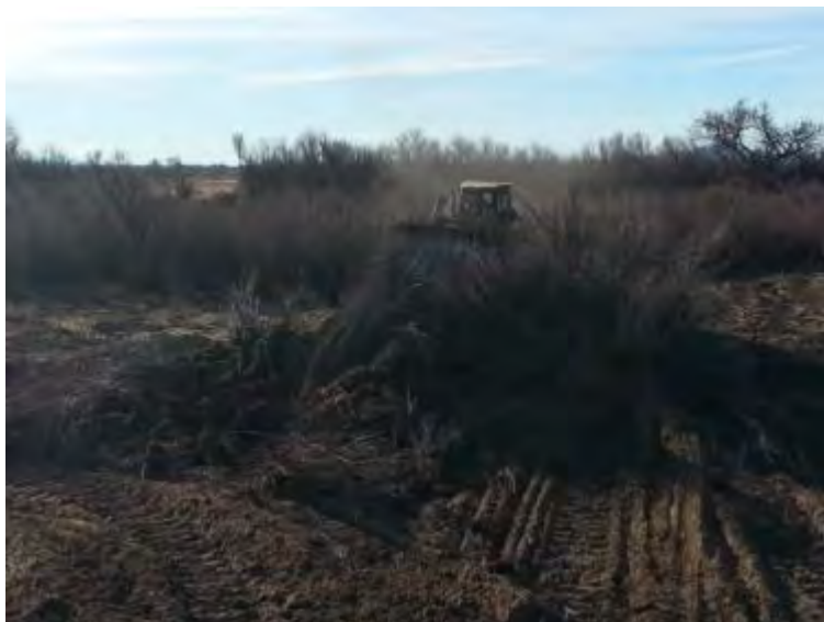
Bulldozer flattening and piling Salt cedar, February 2016
