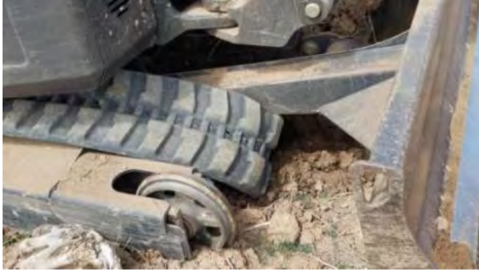
Salt cedar stuck in the tracks sometimes causes them to come off.
