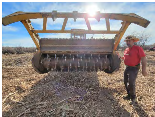
Close up of the masticator head.
